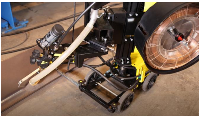
Versotrac Cadet is the ideal tractor for fillet welds.
