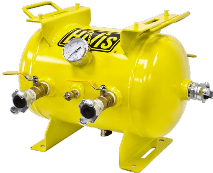
**5 Gallon 4 Port HiVis Manifold.** Eliminate clutter by running just one air hose to your worksite and connect up to eight pneumatic tools at once. Equipped with a gauge to monitor working pressure and a 200 psi pressure relief valve to prevent excess pressure build-up. Top and bottom brackets allow for easy stacking or mounting to skids or other surfaces. Connect or stack multiple manifolds to handle the busiest worksites.
