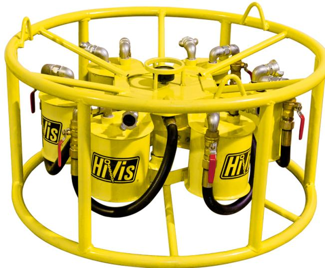
**6 Port Manifold with Moisture Separators.** Ideal for rental, industrial, bridge work, construction, shipyards and demolition industries; anywhere you need to deliver air to multiple users. The 1-1/2" air inlet delivers air through up to six separate outlets with CP fittings. Each outlet has a manual shut-off valve and moisture separator with auto drain valve, increasing tool life. Rugged steel tubular design can be rolled to the jobsite and tabs allow the unit to be lifted and stacked.
