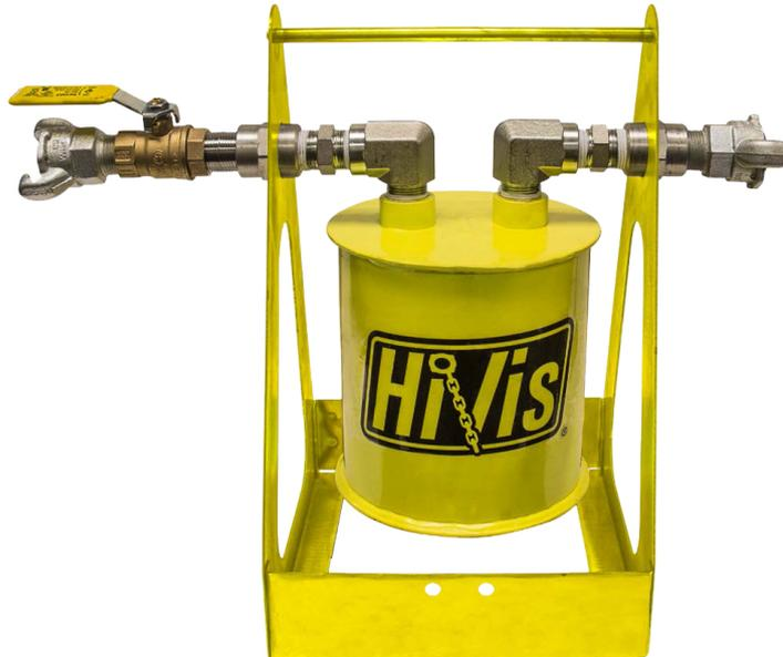
**Moisture Separator - Hand Carry with Automatic Drain.** The HV-S7F-CARRIER moisture separator removes 100% of visible moisture from air lines. It is constructed of high strength steel and features an auto drain valve. This water separator is a portable design that delivers clean air in the most confined and remote places. Minimal maintenance required.
